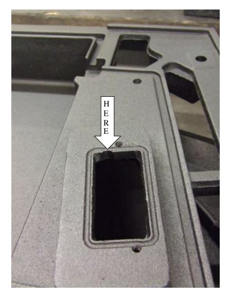
11. Place the pre-cut, *cement free* gasket on the bottom side of the new pilot assembly. Make sure you run each connector through the correct hole.
